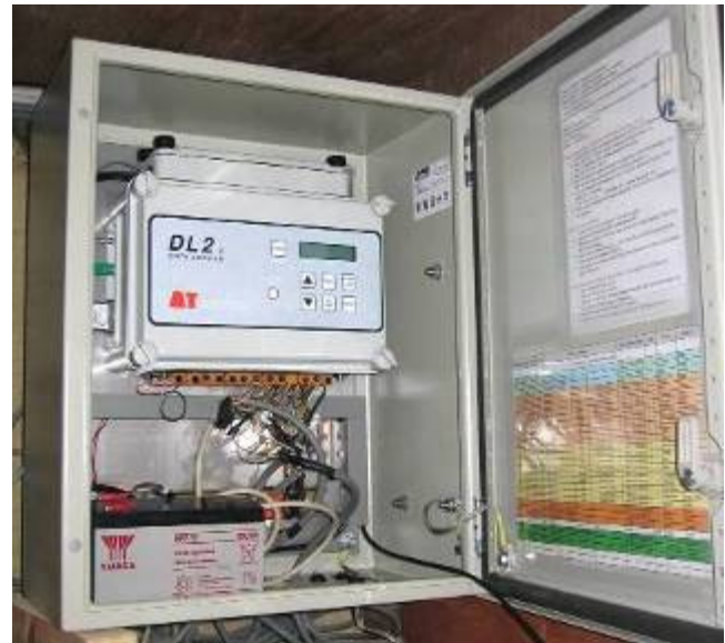
Figure 15 (left): The external weather station sensors (Durabuild, 2004). Figure 16 (right): the datalogger housed in the kitchen (Durabuild, 2004).
